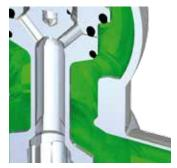
**Open** Valve open Leakage chamber closed
