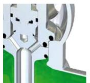
Movement of lower plate Lower line open Leakage chamber closed
