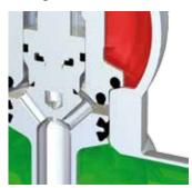
**Closed** Lower valve disc radial seal (RSC seal)
