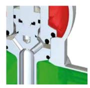
**Closed**Lower valve disc with conical seal
